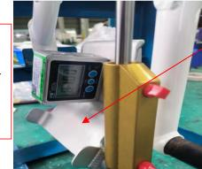
foot pedal installation Angle is  $81{\pm}0.5^{\circ}$
